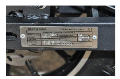
PIN is stamp marked on an aluminum plate that is riveted on the rear swing arm. PIN means the Product Identify Number which is unique for each unit.
