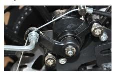
If the brake has too much slack, loosen the rear anchor bolt with a L-wrench and pull the brake wire tighter. The distance of the brake wire between the end of the cable and the anchor bolt should be between 37mm and 44 mm.
