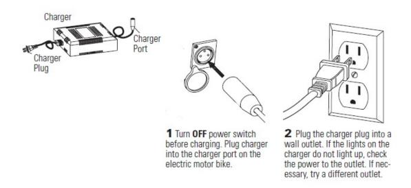
**Warning:** Failure to recharge the battery at least once a month may result in a battery that will no longer hold a charge.
