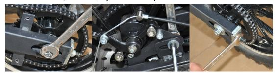
**Step 3:** The chain tension is in good condition while the gap is about 5mm between chain to lowest parts of swing arm. Lock all the nuts and screws, check the wheel alignment and then re-attach the chain cover.
