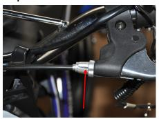
To adjust the brake tension, thread the brake lever adjuster in or out 1/4 or 1/2 turn until the required brake adjustments is attained.
