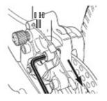
2 Locate the rear brake caliper and disk brake behind the right rear wheel. The distance of the brake wire between the end of the cable and the anchor bolt should be between 37 and 44 mm. If the rear brake has too much slack, loosen the rear anchor bolt with a hexagonal wrench and pull the brake wire tighter (direction indicated with arrow).
