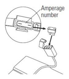
Remove any fuse that is damaged or burnt out and replace with a new one of equal amperage.
