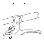
1 To adjust the play, thread the brake lever adjuster in or out 1/4 to 1/2 turn until the desired brake adjustment is attained. Most adjustments are complete at this step. If brake still needs further adjustment, proceed to step 2 for rear brake.
