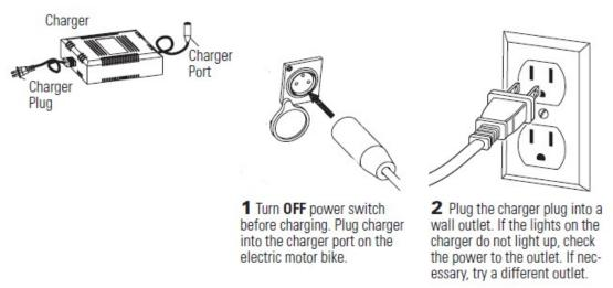
**Warning:** Failure to recharge the battery at least once a month may result in a battery that will no longer hold a charge.
