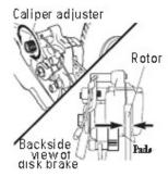
3 If the brake rotor is dragging on the brake pads use your fingers to twist the caliper adjuster in either direction until rotor is centered between pads.
